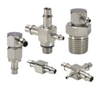
Minimatic® barb fittings provide a flexible, easy alternative to ferrule and push-to-connect design fittings. Electroless nickel plating provides corrosion resistance in applications involving high moisture. Nitrile gasket included with #10-32 threads except when ordered in bulk.
