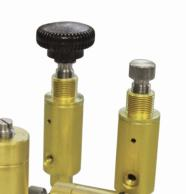
Regulators are offered in either relieving or non-relieving versions. The relieving design maintains a constant pressure output even when downstream conditions change, while non-relieving regulators do not automatically compensate for changes in downstream flow or pressure. There is no vent to atmosphere, as in a relieving type regulator, and the output pressure can increase due to a downstream event. Non-relieving versions can accommodate compatible liquid applications.
